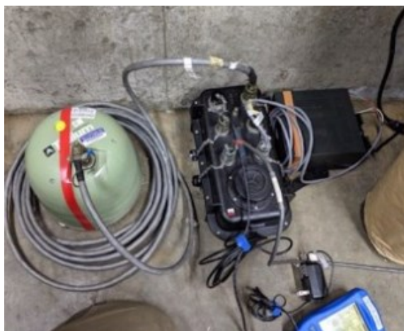
Image: seismometers used to map the basin's shape and contents Source: Pacific Northwest Seismic Network
