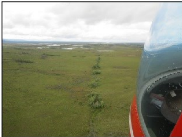
Image: Figure 17. View to the southwest along the Kaltag fault where it projects along the northern flank of the Kaiyuh Mountains toward the Yukon River floodplain. The trace of the fault is marked by pingos aligned with trees through the center of the photo. Photo taken from GPS coordinate 64.457867°, -157.520967°.
