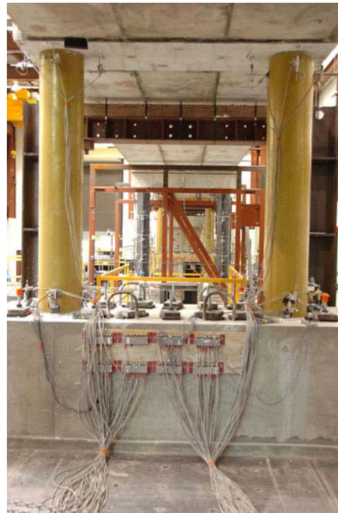
The 200-ton, four-span bridge was built over several months atop the 14-foot-square shake tables at the large-structures lab. The innovative bridge was hit with nine increasingly more powerful earthquakes over several days, and survived. – CREDIT:UNR
